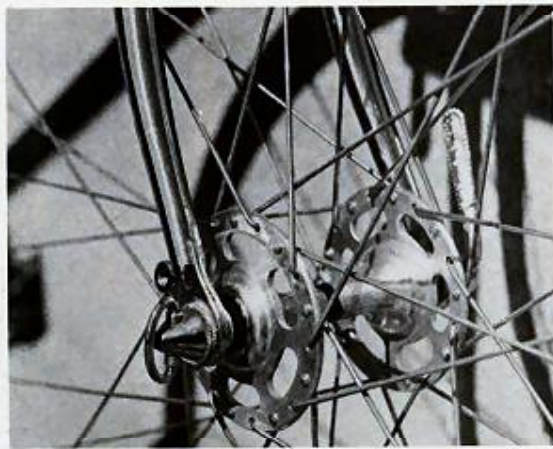
Eyelets have been left on the Campagnolo fork tips to allow easy fitting of racks for touring.
