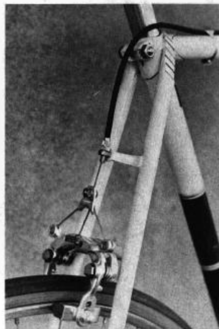
A bridge, brazed to the rear stays, supports the rear brake cable housing stop.
